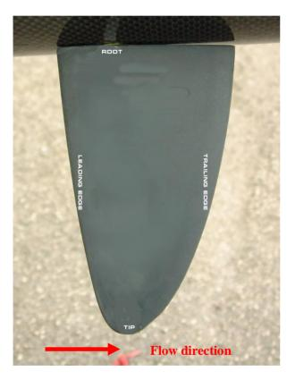
Leading edge – the front, highly curved part of the rudder that makes contact with undisturbed water first
